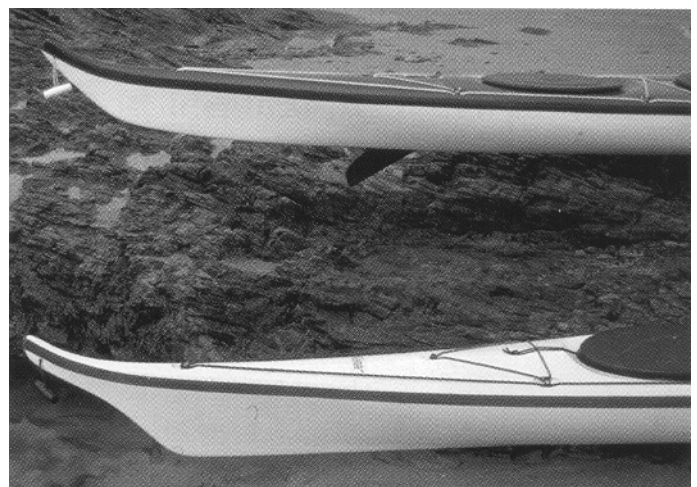
Figure 3) A single change on the hull can totally change the handling characteristics of the boat. Top boat; Nordkapp H, Bottom boat; Nordkapp HM.
