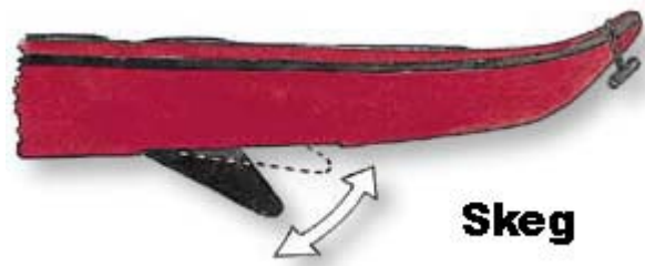
Figure 2) Retractable skeg are available on some kayaks.
